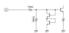
Standby pin internal equivalent circuit diagram
