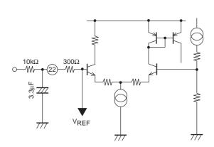
Muting pin internal equivalent circuit
