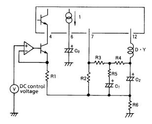
The other problem is that vertical linearity chages when used at multi-frequency (e.g. 40 to 80Hz).
