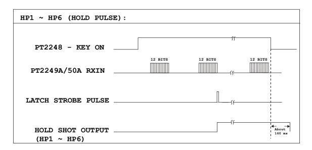
Under abnormal conditions where intolerable interference of any kind would cause the receiver to receive only one matched code word during the last transmission (please refer to the diagram above), then approximately 160 ms after the key is released and the hold shot output (continuous signal) is stopped, the output is reversed to "L" level.
