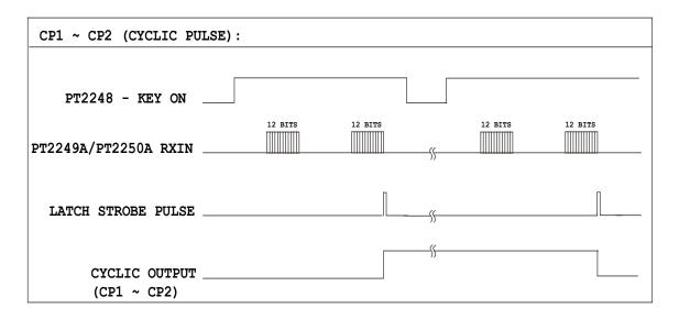
When signal is received, the cyclic pulse output is reversed. This cyclic pulse is used for Power ON/OFF, MUTE, etc.
