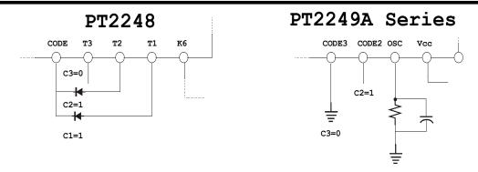
Example 1 Circuit Diagram when Code Bit C2 = 1 and C3 = 0
