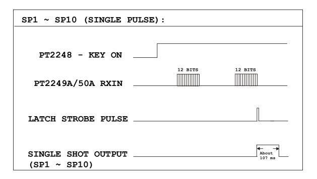
If there is no error in the receiving signal of the 12-bits data check, it will generate a single pulse output.
