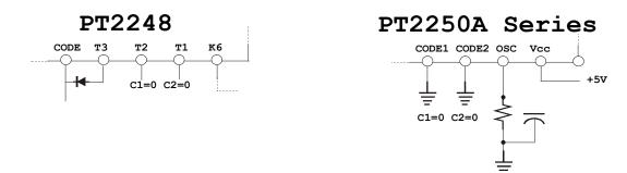
Example 2 Circuit Diagram when Code Bit C1=0 and C2=0
