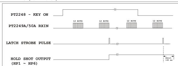
Normally, after two matched code words (12-bits per word) transmitted from PT2248 is detected, the latch strobe is generated, thereby producing a latch strobe pulse. This causes an "H" state output and this output is sustained at "H" level as long as the continuous signal received. Approximately 160 ms after the key is released and the continuous signal is stopped, the output is reversed to "L" level by above. the last latch strobe pulse. Please refer to the diagram
