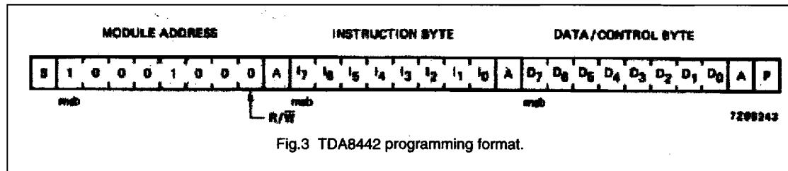
Acknowledge (A) is generated by the TDA8442 only when a valid address is received and the device is not in the power-down-reset mode ( $V_P > 8.5$  V (typ.)).
