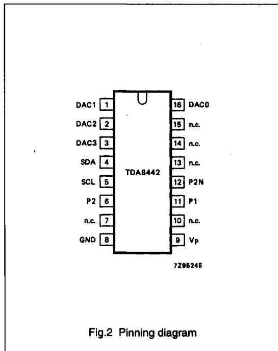
Fig.2 Pinning diagram
