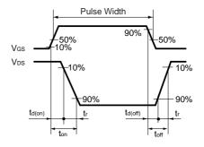
Fig.11 Switching Time Waveforms
