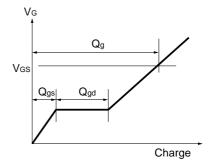
Fig.13 Gate Charge Waveform
