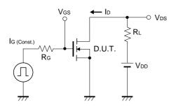
Fig.12 Gate Charge Test Circuit
