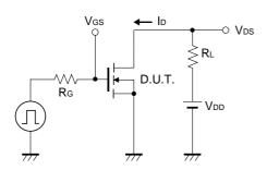
Fig.10 Switching Time Test Circuit
