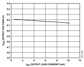
Figure 9. Typical Isolated V<sub>ISO</sub> Output Voltage vs. I<sub>ISO</sub> Output Load Current
