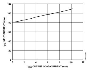
Figure 8. Typical I<sub>DD</sub> Input Current vs. I<sub>ISO</sub> Output Load Current
