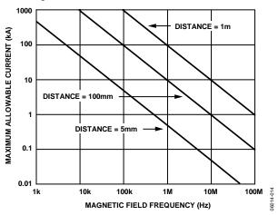
Figure 14. Maximum Allowable Current for Various Current-to-ADuM524x Spacings
