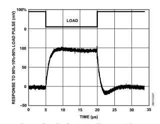
Figure 10. Typical V<sub>ISO</sub> Transient Load Response, 5 V Output, 90%-10%-90% Pulsed Load, 100 nF Bypass Capacitance vs. Time
