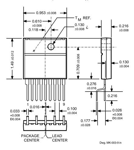
$\label{eq:NOTE:exact body and lead configuration at vendor \~Os option within limits shown.}$
