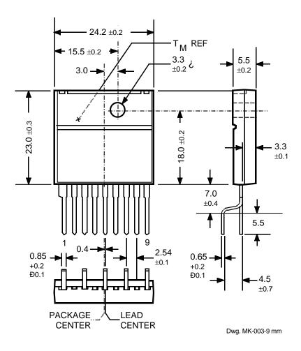
NOTE: Exact body and lead configuration at vendorÕs option within limits shown.
