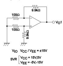
3. Common-mode signal rejection ratio [CMR] Common-mode input voltage range  $[V_{ICM}]$
