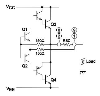
In source mode, when Q3 turns on and current flows into the load resistor, a voltage difference occurs across RSC, turning on Q1 and activating the current limiter.
