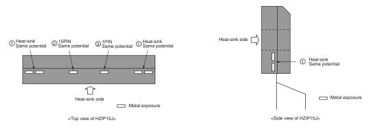
• Frame diagram (LV5680NPVC) \*In the system power supply other than LV5680NPVC, pin assignment may differ.
