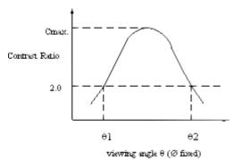
Remark: Optimum viewing angle with the naked eye and viewing angle 8 at Cmax
