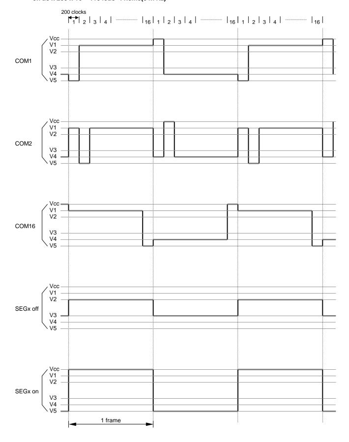
Assume the oscillation frequency is 270KHZ, 1 clock cycle time = 3.7us, 1/11 duty; 1/4 bias,1 frame = 3.7us x 400 x 11 = 16280us=16.3ms (61.3Hz)
