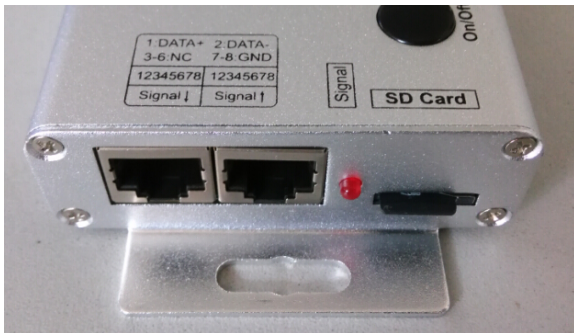
Signal input - network card holder and small SD card socket
