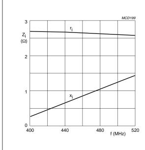
Class-B operation;  $V_{CE}$  = 7.5 V;  $P_L$  = 8 W.
