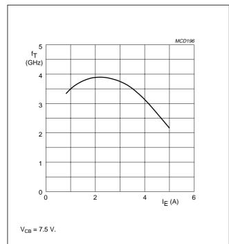
Fig.6 Transition frequency as a function of emitter current, typical values.
