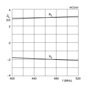
Class-B operation;  $V_{CE} = 7.5 \text{ V}$ ;  $P_L = 8 \text{ W}$ .
