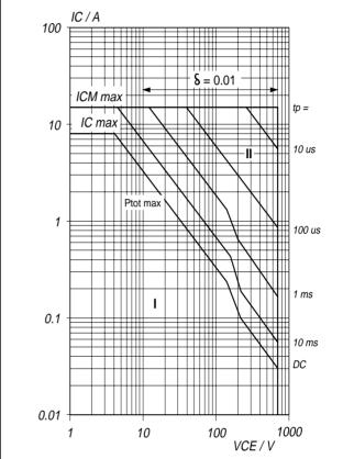
Fig.11. Forward bias safe operating area.  $T_{hs} = 25\,^{\circ}\text{C}$  l Region of permissible DC operation. Il Extension for repetitive pulse operation.
