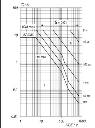
Fig.10. Forward bias safe operating area.  $T_{hs} = 25^{\circ}C$  l Region of permissible DC operation. Il Extension for repetitive pulse operation.
