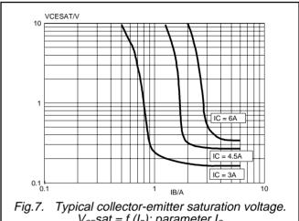
Typical collector-emitter saturation voltage.  $V_{CE}$ sat =  $f(I_B)$ ; parameter  $I_C$
