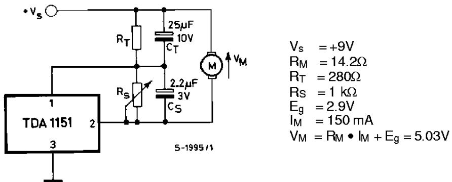
Note: A ceramic capacitor of 10 nF between pins, 1 and 2 improves stability in some applications.
