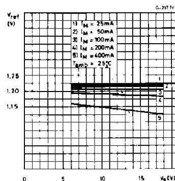
**Figure 4. Reference voltage vs. motor current**
