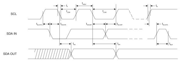
Figure 6. Write Cycle Timing
