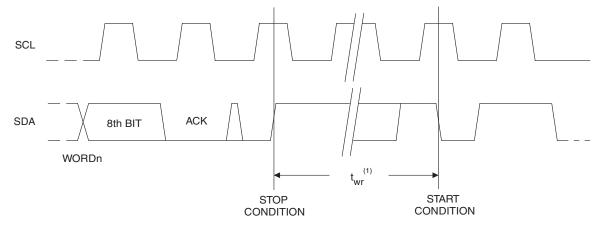
Note: 1. The write cycle time t<sub>ws</sub> is the time from a valid stop condition of a write sequence to the end of the internal clear/write cycle.
