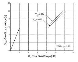
Figure 6. Gate Charge Characteristics
