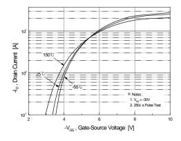
Figure 2. Transfer Characteristics
