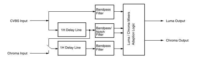
Fig. 2-2: Block diagram of the adaptive comb filter (PAL mode)
