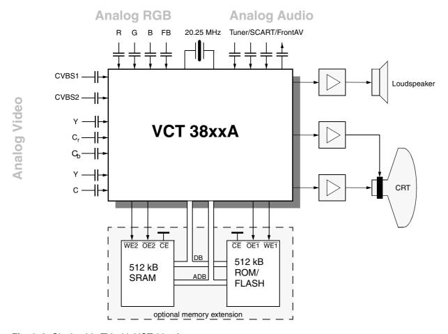
Fig. 1-3: Single-chip TV with VCT 38xxA
