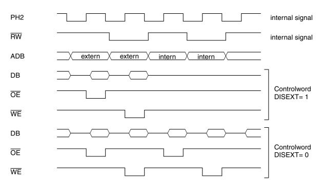
Fig. 5-2: Internal/external memory access
