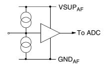
Fig. 6-10: Input pins VIN1-VIN4
