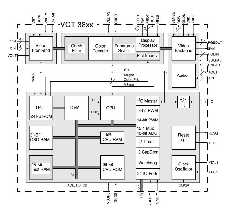
Fig. 1–2: Block diagram of the VCT 38xxA (shaded blocks are optional)
