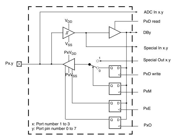
Fig. 5-5: Universal port circuit
