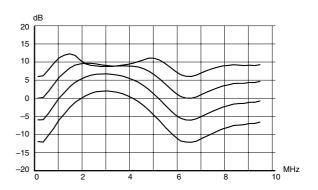
Fig. 2-13: Dynamic peaking frequency response
