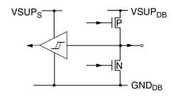
Fig. 6-31: Input/Output pins DB0-DB7
