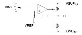
Fig. 6–13: Output pin VOUT
