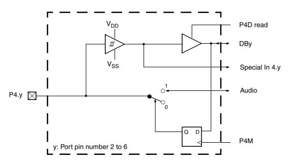
Fig. 5-7: Audio port circuit
