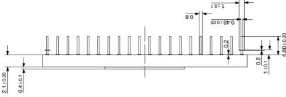
Fig. 6–3: 257-Pin Ceramic Pin Grid Array (CPGA257)
