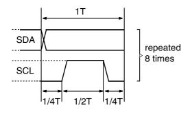
Fig. 5–20: Single bit on I<sup>2</sup>C bus
