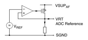
Fig. 6-14: Supply pins VRT, SGND
