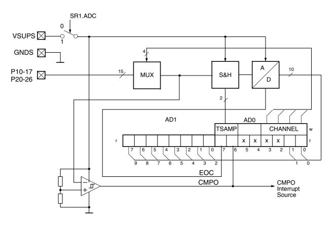
Fig. 5-4: Block Diagram of the ADC
