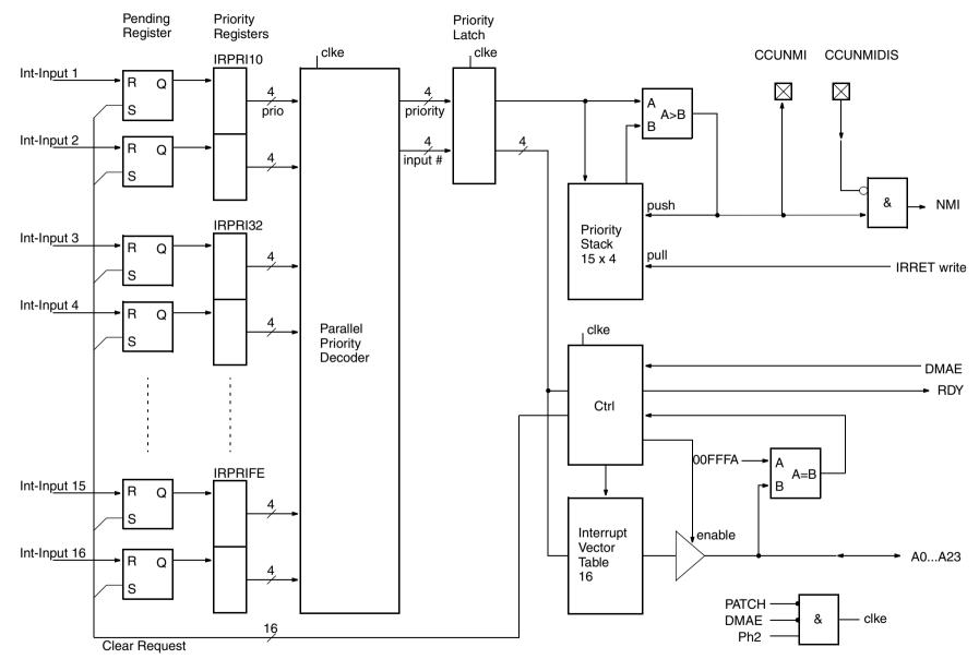
Fig. 5–10: Block diagram of interrupt logic
