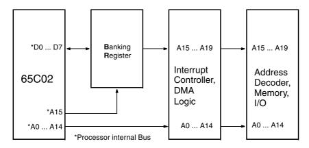
Fig. 5-5: Block diagram of Memory Banking
