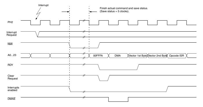
Fig. 5-15: Interrupt timing diagram
