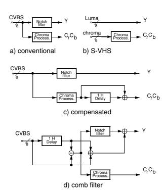
Fig. 2-6: NTSC color decoding options
