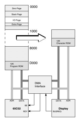
Fig. 3-2: Memory environment of text controller
