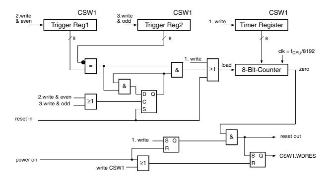
Fig. 5-4: Block diagram of watchdog
