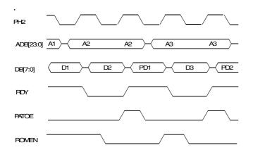
Fig. 5-17: Patch timing
