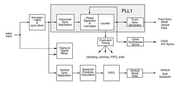
Fig. 2-10: Sync separation block diagram
