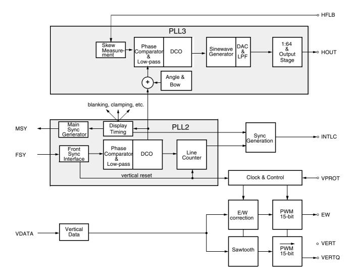
Fig. 2-24: Deflection processing block diagram
