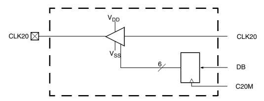
Fig. 5-8: CLK20 Port Circuit
