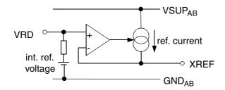
Fig. 6-25: Supply pins XREF, VRD
