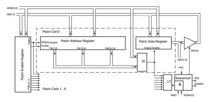
Fig. 5-16: Block diagram of patch module
