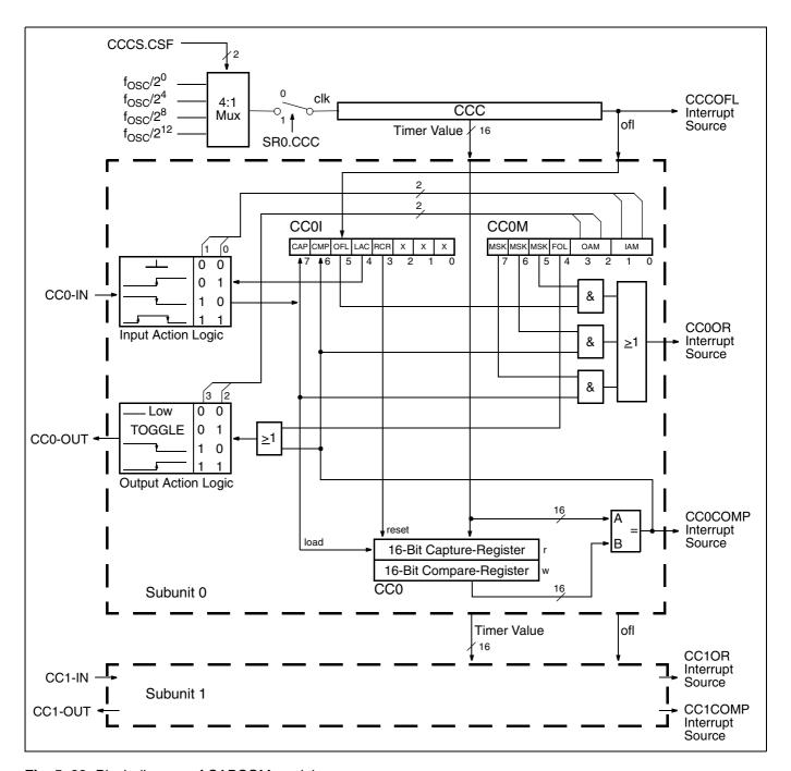
Fig. 5-23: Block diagram of CAPCOM module
