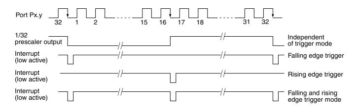
Fig. 5-14: Interrupt timing (1/32 Prescaler On)
