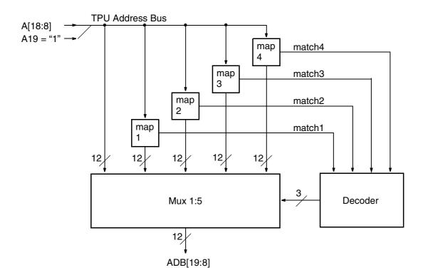
Fig. 5-8: DMA address mapping
