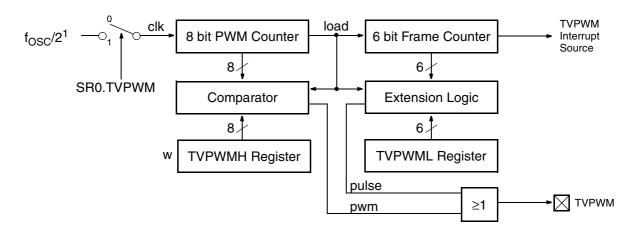
Fig. 5-2: Block Diagram of 14bit Tuning Voltage PWM
