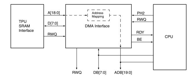
Fig. 5-7: Block diagram of DMA interface
