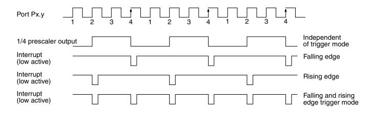
Fig. 5–13: Interrupt timing (1/4 Prescaler On)
