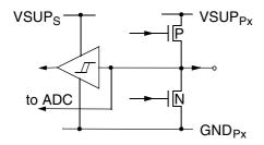
**Fig. 6–28:** Input/Output pins P10-P17, P20-P27, P30-P37
