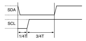
Fig. 5-21: Stop condition I<sup>2</sup>C bus
