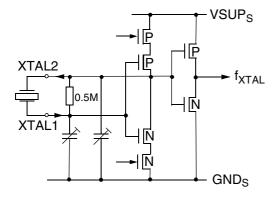
Fig. 6-8: Input/Output pins XTAL1, XTAL2
