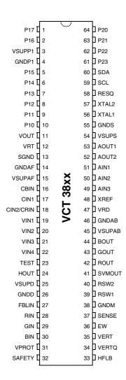
Fig. 6-4:64-pin PSDIP package
