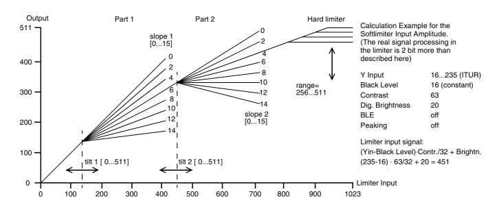
Fig. 2–15: Characteristic of soft limiter A and B and hard limiter
