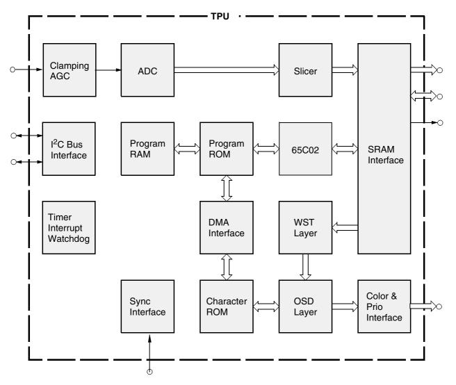
Fig. 3-1: Block diagram of the TPU
