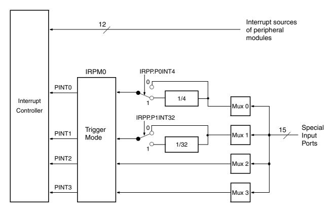
Fig. 5-12: Interrupt assignment and multiplexer
