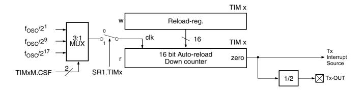
Fig. 5-22: Block diagram of timer T0 and T1
