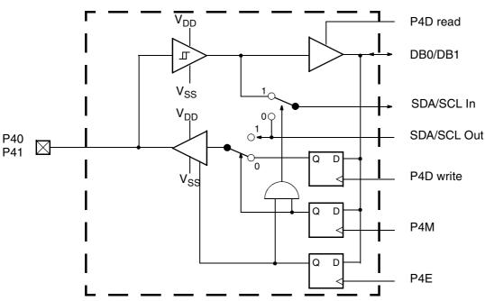
Fig. 5-6: I<sup>2</sup>C port circuit
