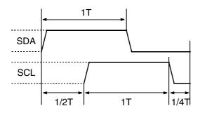
Fig. 5-19: Start condition I<sup>2</sup>C bus
