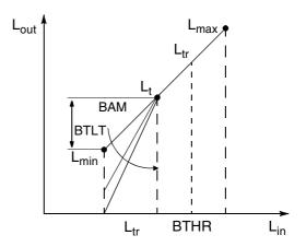
Fig. 2–11: Characteristics of the black-level expander
