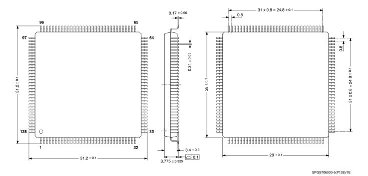
**Fig. 6–2:** 128-Pin Plastic Metric Quad Flat Package **(PMQFP128)** Weight approximately 5.4 g
