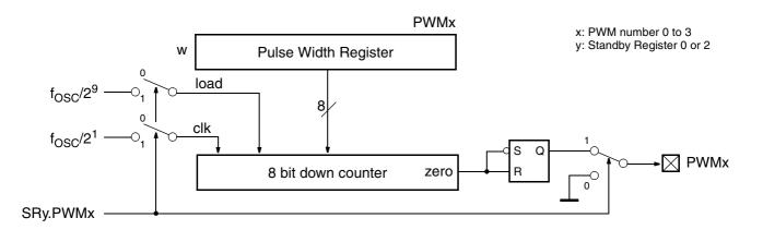
Fig. 5-1: Block diagram of 8-bit PWM
